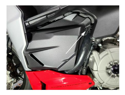
3. Slide Fuse/Battery cover backwards to remove the Fuse box and battery.
