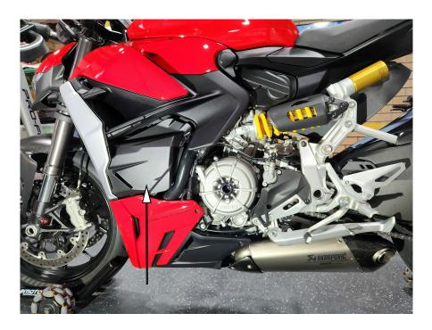
2. Using a 3mm Allen key wrench, remove the single screw holding on the Fuse/Battery cover
